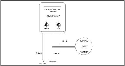
The XPFM Incandescent and Inductive Non-dimming Fixture Module is designed to control 15A loads ON and OFF. The XPFM is small enough to fit inside recessed lighting cans and single gang boxes of new or existing loads, allowing hard wired control from inside the fixture.
