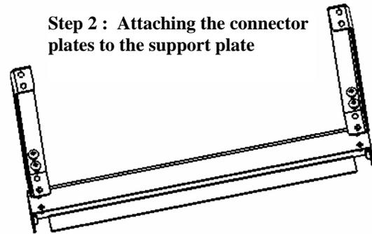
2. First attach the connector plates (#10) to the support plate A (#4A) using the 1/4" – 20UNC screws (#7).
