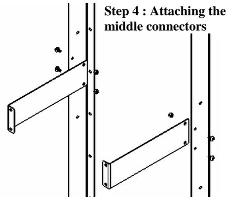
4. Attach the middle connector plates (#11) to the left and right "L" supports (#2A and #2B) using the 1/4"- 20 screws and nuts (#7 and #8).
