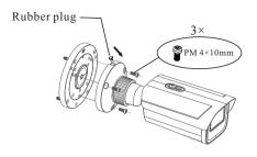
⑤ Connect the cables and then install the camera onto the junction box as shown below.
