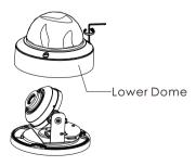
③ Route and connect the cables. Then secure the camera to the ceiling or wall with the screws provided.
