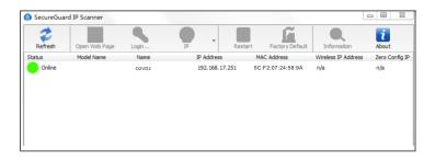
③ In the device list, you can view the IP address, model number, and MAC address of each device. Select the applicable device and double click to open up the web viewer. You can also manually enter the IP address in the address bar of the web browser.
