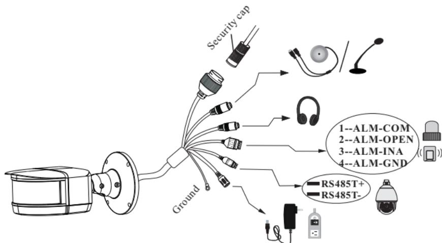
\* 1 It is recommended to install the security cap for outdoor installations.
