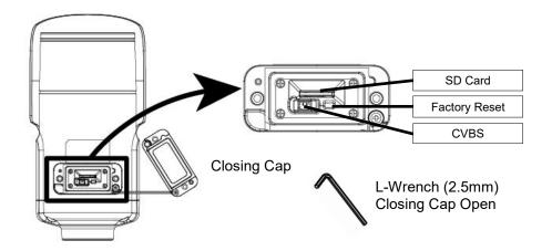
**X** Open the Closing Cap and fasten the Closing Cap well.
