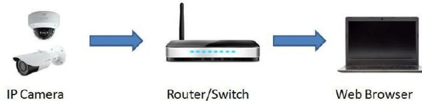
① Make sure the PC and IP-Cam are connected on the same local network. The camera is set to DHCP by default and will be assigned an IP address by the DHCP server. Make sure that the local network has a DHCP server. Routers typically have a DHCP server built in.
