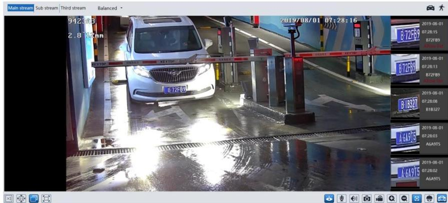
When the captured license plate is matched with the license plate of the comparison list, the list type will be displayed under the license plate number. Click the matched license plate picture, the matched details will pop up as shown below.
