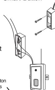
5. If the wall button wires are hidden inside the wall, please connect the "Easy Clip™" to the exposed wires attached to the terminals of the garage door opener.
