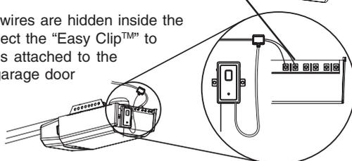
6. Power up the garage door opener, the red LED on the Smart Button™ GB-318 should keep flashing slowly for 2 minutes.
