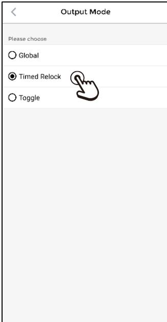
Click *Timed Relock* override the *Output Mode (Global)* or to give the user a different *Output Time* setting if the global mode is *Timed Relock*.
