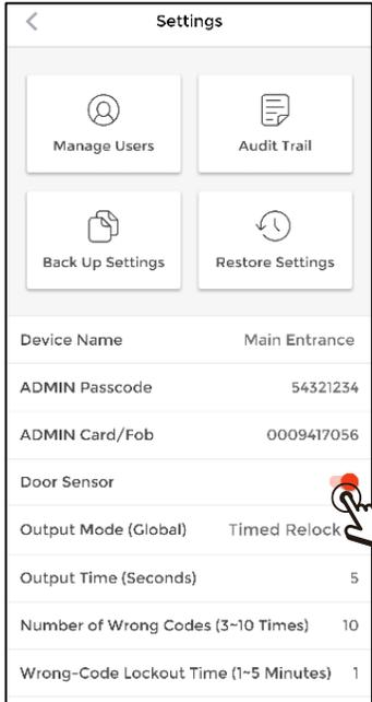
Enable the door sensor\* for a warning when the door is held open longer than the set relock time (see pg. 15) or if the door is forced open. Note that the device cannot distinguish between a door forced open and a door that is held open beyond its relock time.
