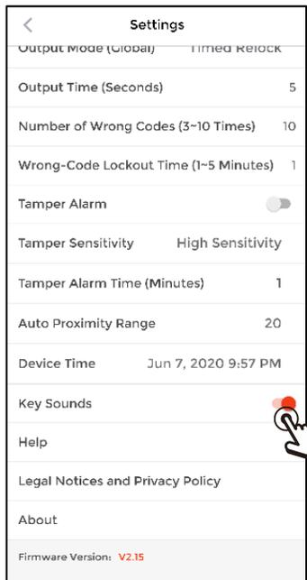
Enable the key sounds for an audible indicator when the keys are pressed.†
