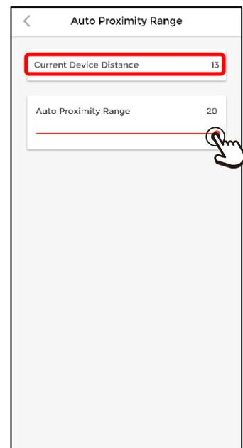
Note that the *Current Device Distance* is also shown on this screen. Use the slider to adjust your *Auto Proximity Range* to a number that closely matches the *Current Device Distance*.
