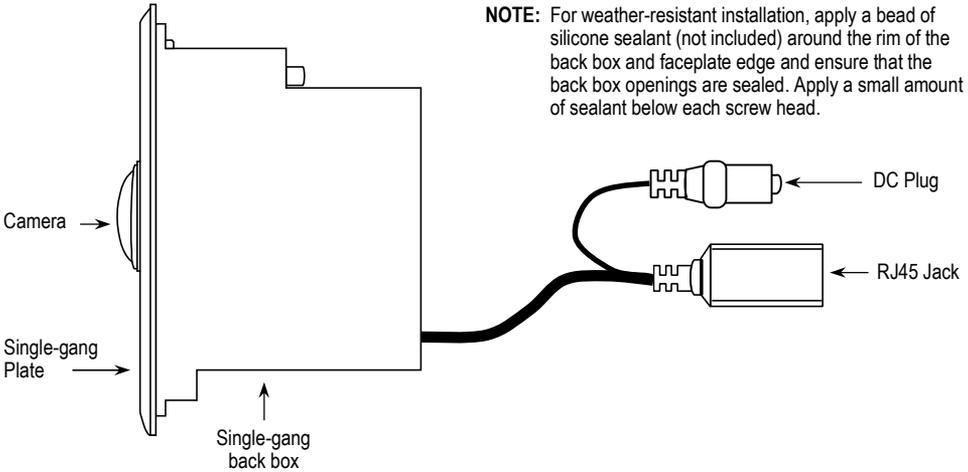
**NOTE:** For weather-resistant installation, apply a bead of silicone sealant (not included) around the rim of the back box and faceplate edge and ensure that the back box openings are sealed. Apply a small amount of sealant below each screw head.
