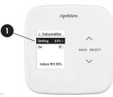
Use the dehumidification adjustment to set the dehumidification setpoint to 60% when first installed. Allow dehumidification to run until the initial setpoint is reached, before deciding if you want to change the humidity setting.
