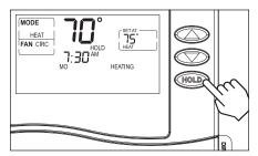
Press (HOLD) to permanently hold the temperature at its current setting. This will override the temperature settings for all time periods of the programmed schedule. With the thermostat in permanent override, the thermostat temperature can be manually adjusted and will stay at that setting until the override is cancelled.
