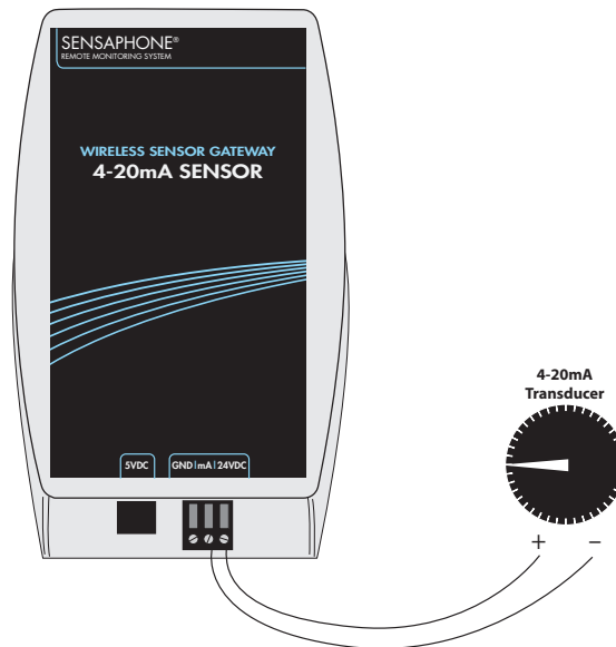
4-20mA Transducer using 24VDC power supply
