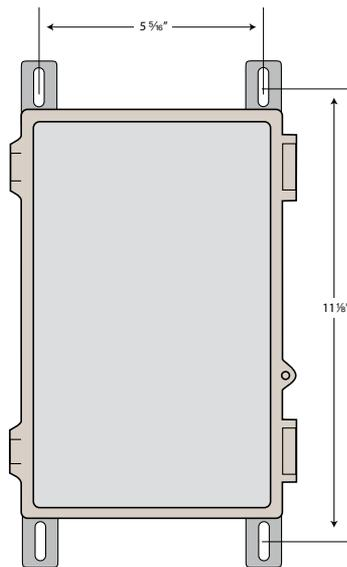
Figure 1: Mounting Dimensions
