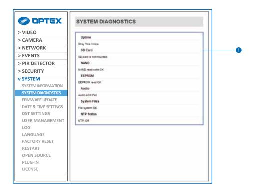
Shows basic hardware functions after inspection.
