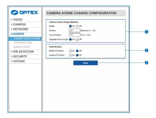
The Camera Scene Change Detection feature is intended to detect camera tampering events such as bagging, defocusing and moving the camera. This is achieved by detecting large persistent changes in the image.
