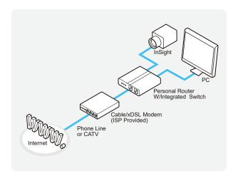
Case B: Static(Fixed) IP + Personal Router [Efficient]
