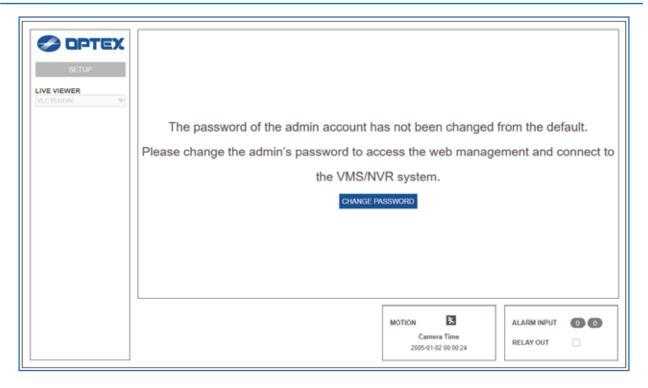
Password change is required at initial connection in factory reset state.
