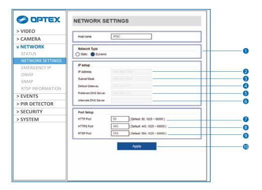
Network Type - Define network IP address type from the Static Mode for the fixed IP or the Dynamic Mode by the dynamic IP address.
