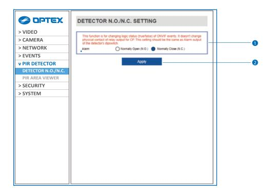
1 Input Device Setup - Select input device type from N.O. / N.C.
