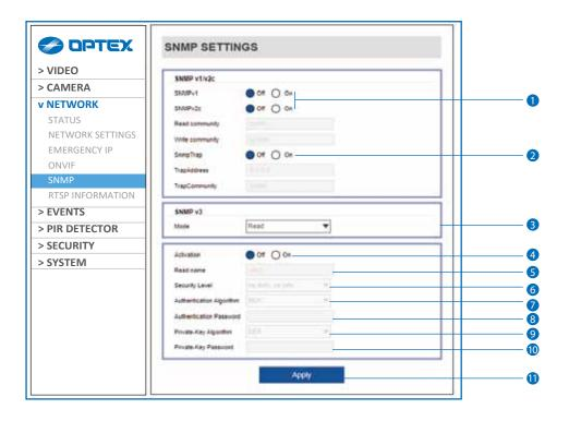
**1 SNMPv1/SNMPv2 -** Select the SNMPv1/SNMPv2 option and type the names of Read community and Write community.
