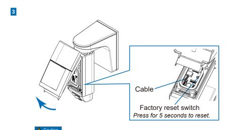
Do not pinch the cable when restoring the PIR detector.
