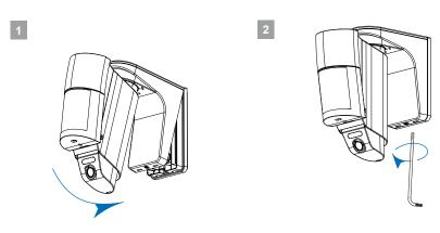
Do not pinch the cable when restoring the PIR detector.
