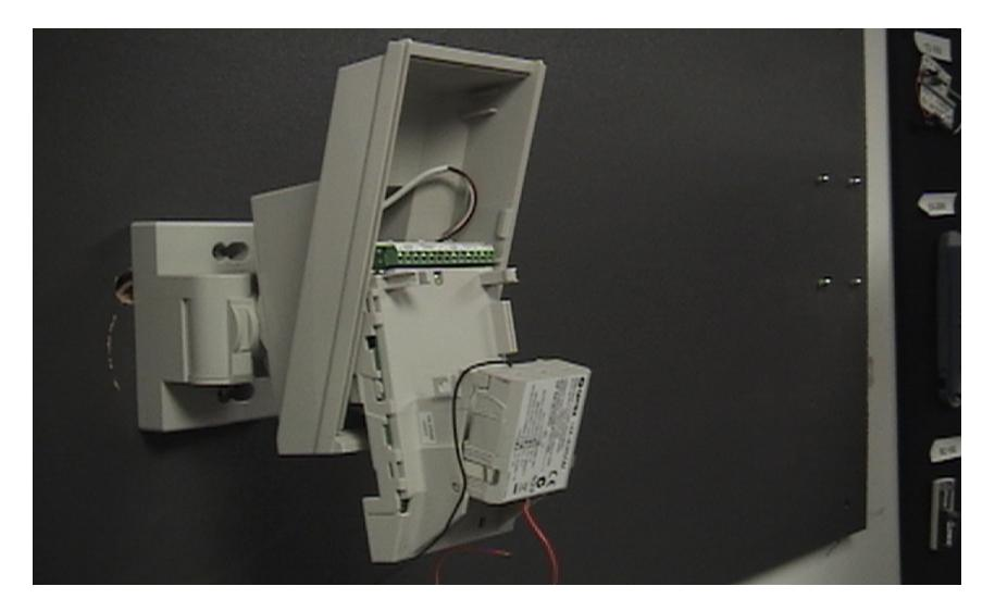
If you are **Not Battery Sharing**, you will need to provide batteries to power both the HX40RAM and the transmitter.
