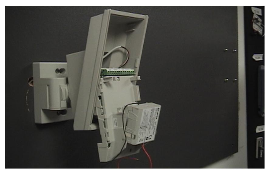
Remove the Battery case by grasping the claws on each side and pulling straight out from the main unit. Now you are ready to install batteries!
