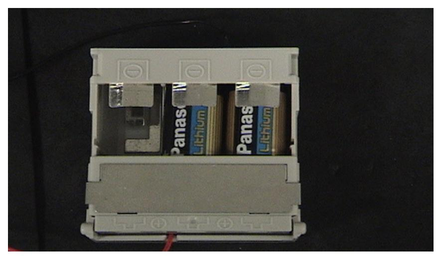
When Not Battery Sharing: Use 3 of each: CR123A or CR2's Do not use ½ AA batteries.
