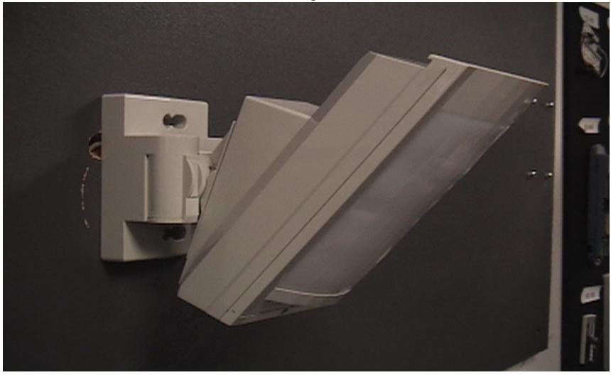
Or you may adjust it for an upward slope. (Do not change the detection range with the bracket, use
