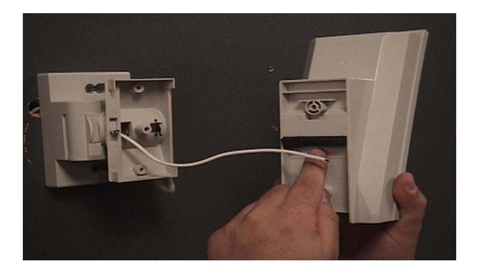
Then replace the Sponge! Next, Install the adjustment screw. Be sure not to tighten too much to be able to adjust the detector. Once adjusted, then tighten the screw.
