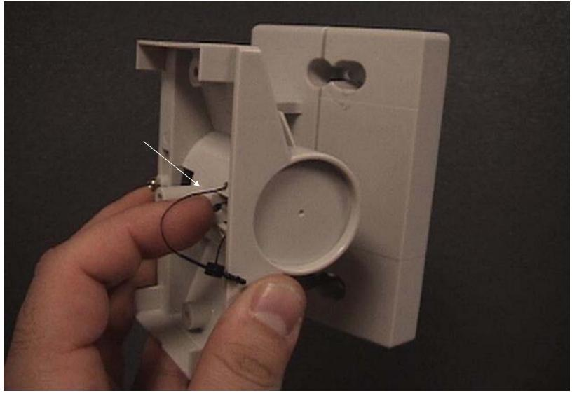
Loosen the screw to open the Bracket. Note, there are two ways to install the Bracket. 90 degrees to the right, or....
