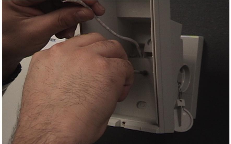
For convenient access to terminals, the detector can be placed facing toward the housing by the tabs on the side
