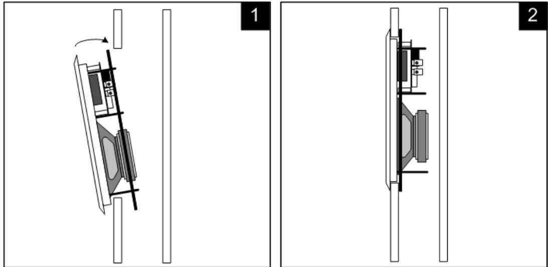
speakers to be placed will not be obstructed by a stud or other material hidden in the wall. Proper use of an electronic stud-finder is invaluable for this operation. Using the proper equipment, cut the appropriate sized hole in the wall. On drywall, the cleanest cuts will be made with a drywall saw.
