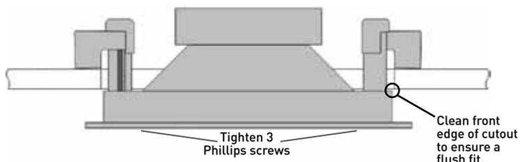
**CAUTION: DO NOT OVER-TIGHTEN THE CLAMPS.** Too much torque may damage the toggle, causing the speaker not to seat securely. A snug fit is all that is necessary to assure proper performance.
