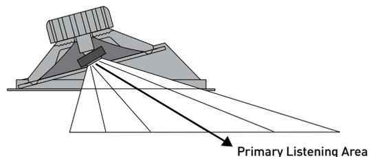
We recommend directing the woofer and tilting the tweeter toward the listening position. **USE CARE TO AVOID DAMAGING THE DOME OF THE TWEETER WHEN AIMING!**
