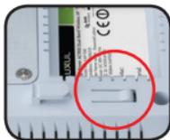
To Reboot the AP: With the XAP-1510 powered on, simply press and release the Reset button.
