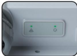
**WLAN:** If the blue LED is On, the wireless radio is active and wireless access is enabled. Off indicates the wireless radio is not active and wireless access is disabled.
