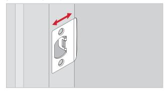
The hole in the door frame for the latch bolt is not drilled deep enough.
