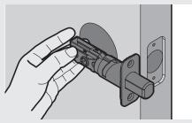
Is the D-shaped hole centered in the door hole?
