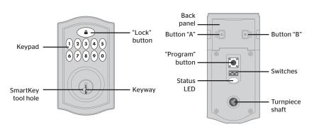
Note: When the cover is removed, the turnpiece shaft can be used to manually lock and unlock the door.
