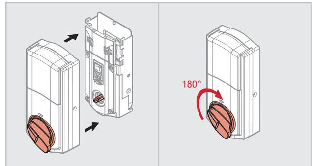
Align the turnpiece with the torque blade and reinstall the interior assembly on the door.
