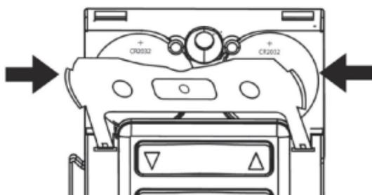
2. Remove the small screw from the battery retainer door. Pull out on the top of the door (it is hinged at the bottom).
