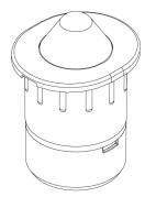
NOTE: The sensor typically protrudes .060" beyond the door jamb. Protrusion may vary slightly.
