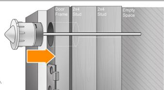
Insert Plunger and Antenna into the door jamb.
