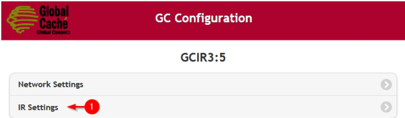
If an IR blaster will be used select Blaster, otherwise select Emitter. Press Apply Changes to save the configuration. All remaining configuration will be done in the chosen control software.
