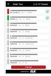
3. Exercise each sensor and verify it is functioning correctly. When testing has been completed, tap the Cancel button.
