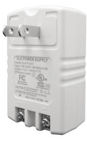
The ELK-P1417 14VDC plug in power supply features built-in overload reset and screw terminals for connections. It is ideal for alarm, access control, and CCTV applications requiring up to 1.7 amps. A receptacle mounting bracket is included.
