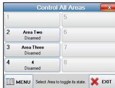
To change the status of any Area while in this mode, simply click on the Area from this screen and the Area will change its state from Arm / Disarm or visa versa. This also allows for multiple Areas to be selected to be changed from the one screen.
