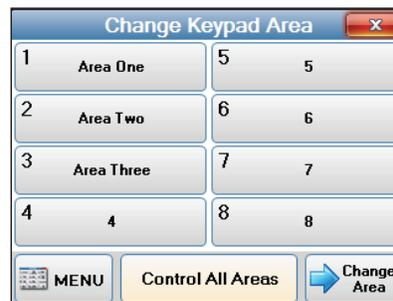
After 1 minute of no key presses the keypad will return to display its primary assigned area.
