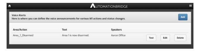
Pressing the test button will simulate as if the M1's event triggered.
