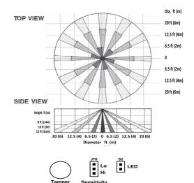
Lo Sensitivity - 3 event - place jumper on top two pins Hi Sensitivity - 2 event - place jumper on bottom two pins LED - jumper installed across pins for visual walk test
