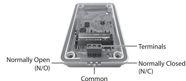
3. After inserting the wires, tighten the terminals with a small screwdriver.
