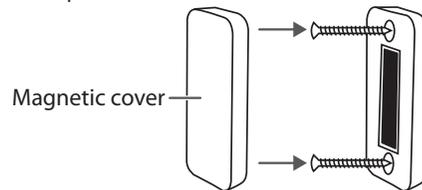
4. Mount the transmitter bracket with a drill and two screws (included). Make sure that the arrow on the bracket is facing up.
