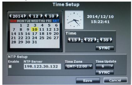
Click the button within the "Time" block for adjusting and synchronize the time of the NVR as the system time of the PC. Moreover, if the user clicks the enable checkbox and the button within the "NTP Setup" block, the time of the NVR will be synchronized as the NTP Server.
