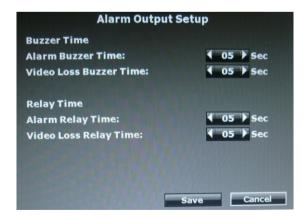
This control item is divided into two parts, "Buzzer Time" and "Relay Time". The user can press? or? to switch the external buzzer time and video loss buzzer time in "Buzzer Time" option. The adjustment value is from 5 to 99 seconds. Moreover, among "Relay Time" option, users can press? or? to switch the external buzzer time and video loss buzzer time. The adjustment value is also
