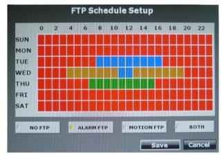
Select the time that the recording video is uploaded to FTP. No file will be uploaded during "NO MAIL" period even the motion detection is triggered.
