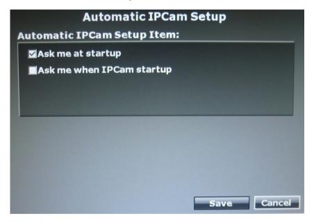
If **Ask me at startup** is ticked, the NVR will activate the **PLUG & PLAY** function to ask for your permission locating any network device within its LAN.
