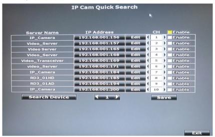
The NVR searches for all the IP devices listed in the LAN. Find the IP camera you want to connect to, assign a channel number for it, and tick "Enable" so for enabling this IP camera and adding it to all-channel list.
