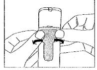
Place the clip against the battery cover and press firmly so that it locks on.
