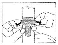
Remove the clip by using the small round handles and pressing out from the sides.
