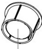
(Magnetic Sensor contains a magnet inside the plastic shell)
