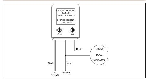
The XPDF Incandescent Dimmer Fixture is designed to control Incandescent loads of up to 300W. The XPDF is small enough to fit inside recessed lighting cans and single gang boxes of new or existing loads, allowing hard wired control from inside the fixture.
