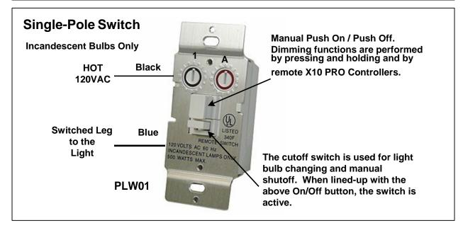
**Description:** The PLW01 Wall Dimmer Switch is designed to control incandescent bulbs (only) with a rating of 40 to 500W. Bulbs rated below 40W may flicker and/or operate erratically. A pushbutton is provided for local On/Off control and manual bright / dimming operation. A Power Cutoff Switch located directly below the Local On/Off Pushbutton is provided for bulb changing. Both switches should line-up for normal operation.
