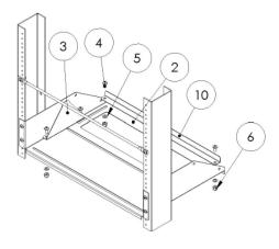
Step 4: Attaching the triangle plates
