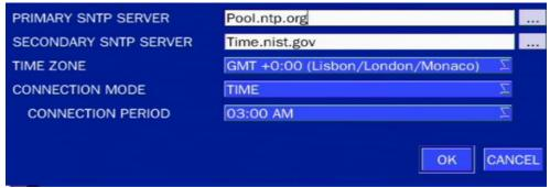
**PRIMARY SNTP SERVER**: Input the address of the primary NTP time-server.
