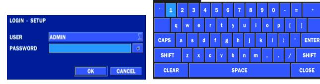
When the DVR prompts the LOG-IN window, enter the PASSWORD using the virtual keyboard, or the remote control. The factory default password is 1111. It is highly recommended to assign a new password to protect the system. New passwords can be set up in the SECURITY setup menu.
