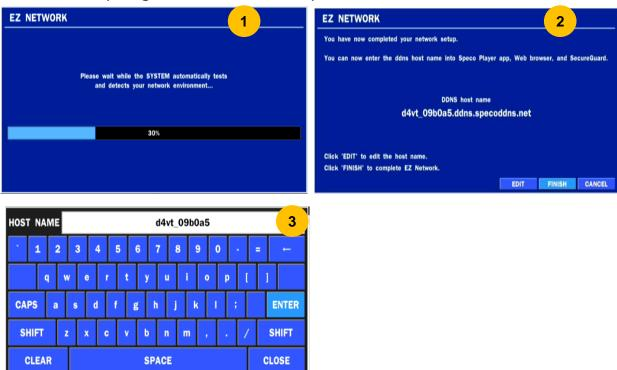
Figure 2.4.2. EZ NETWORK Setup Procedure
