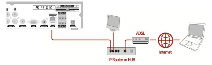
1. Go to SETUP>NETWORK>DDNS and set the DDNS SERVER to ON.
