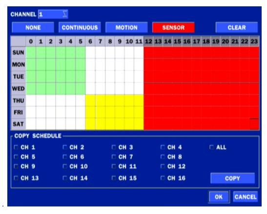
Figure 4.3.2. Schedule Recording Setup Screen
