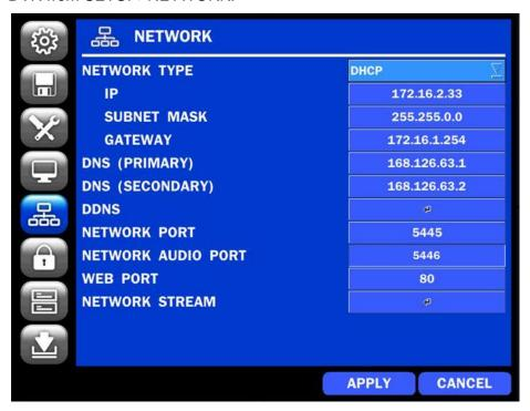
8. Port forward the NETWORK PORT (Default: 5445) and WEB PORT (Default: 80) of the private IP Address of the DVR on the network router.
