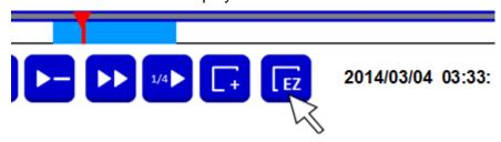
3. Move time bar cursor to the time of end of backup and press EZCOPY button. Then, EZCOPY STOP time will display.
