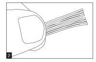
Insert the conductors through the holes in the wire guide making sure to keep them in the proper color code order.
