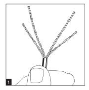
2) Separate pairs and lay out per the T568A or T568B specification required for your application. Use the convenient color chart on the EZ-SnapJack wire guide to assist you.
