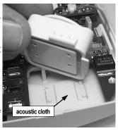
With the acoustic 6 cloth removed, the siren dB level will be consistent with UL Audibility requirements.
