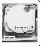
Use a small screwdriver to push the locking clip away 4 from the retaining tab to unlock the Siren Module.
