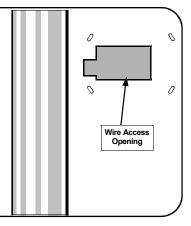
4 Pull wires through access hole
