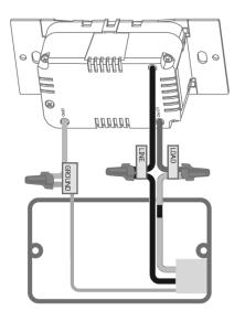
are required for proper operation Note: Line, Load and Ground connections
