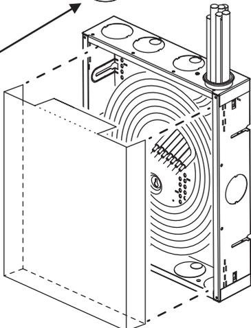
After cabling is routed, reverse paint shield and return it to the enclosure to protect cabling.
