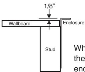
When mounting without using the mounting tabs adjust the enclosure to protrude 1/8" beyond the wallboard surface.
