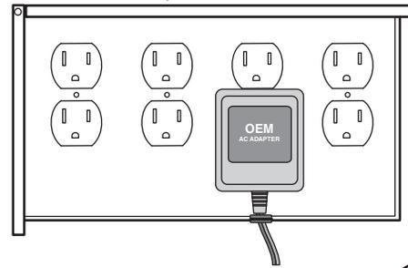
The H290/(H291) provides space for 4/(2) standard duplex receptacles. Wires should exit the H290/(H291) using the grommets provided. The grommets may be cut as shown.
