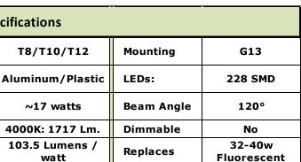
Life Power >90 CRI: 82 Factor: Mercury/ IR / UV None None **Lead Content** 1.17" Warranty 5 year Limited **Dimensions** X 4' nom.
