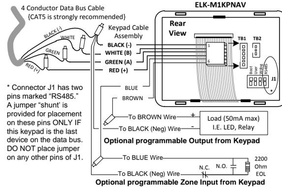
The optional Zone Input # and Output # is determined by the Keypad Address.
