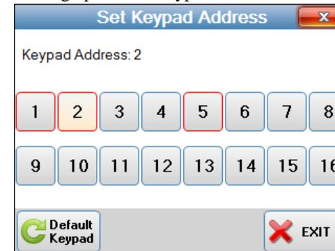
The current keypad address will be illuminated. Any address(s) with a RED border indicate a keypad currently enrolled to the M1 panel. RED bordered addresses **CANNOT** be used for this keypad.
