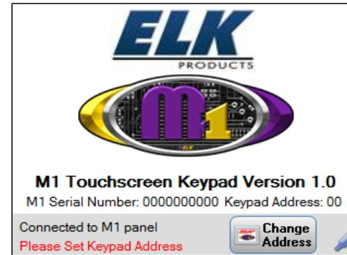
A message along the bottom “Please Set Keypad Address” will display if a keypad address is not currently set. Otherwise the message will display “Waiting to connect to panel”. This displays until Navigator receives valid data from the panel.
