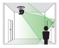
Camera module integration. When video outdoor station is integrated with an analog camera, the field of vision and monitoring range will be significantly enlarged. In addition, residents are free to switch between the inbuilt camera on outdoor station and the additional analog camera for surveillance purpose through cyclic selection among all outdoor stations, no matter in standby or during video conversation with visitors.
